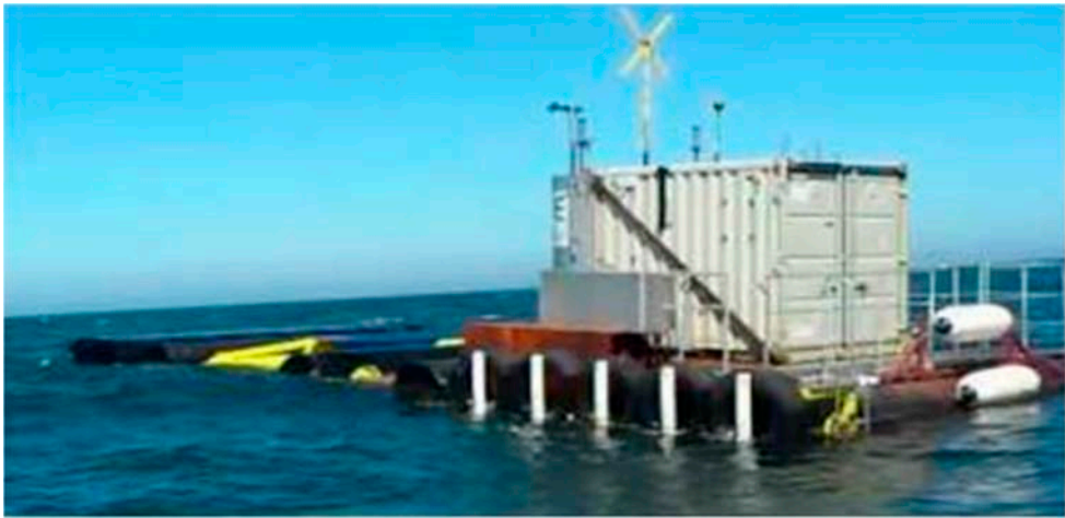
B - Sveifla dufls (e. Point Absorber)
