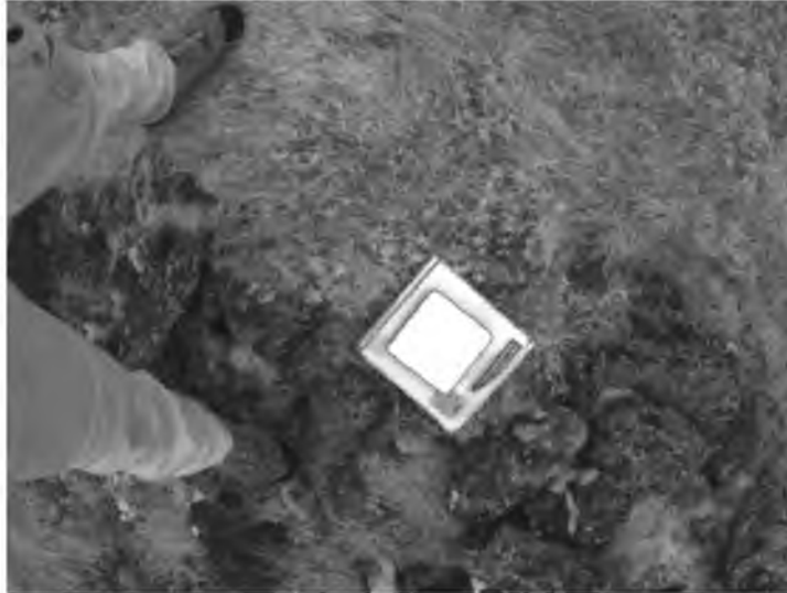
Figure 5. Reflectance target sensed with the NIR sensor. It was sensed for every flight with every sensor used
